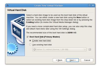
The wizard allows you to create an image file or use an existing one. Note also that the disk images can be separated from a particular VM, so even if you delete a VM, you can keep the image, or copy it to another host and create a new VM for it there.
